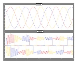
Figure 4 Voltage and current waveform at supply point
