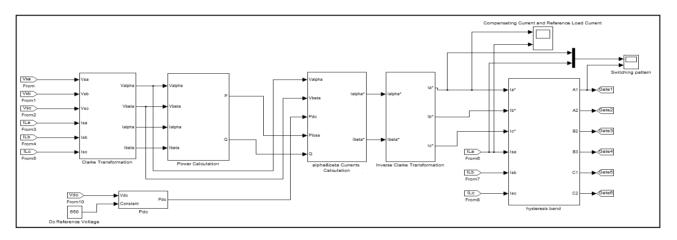
Figure 8 Control circuit for harmonics compensation
