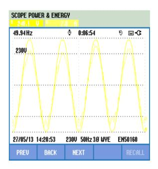
Figure 22 Voltage and current waveform for phase b
