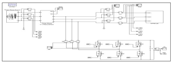
Figure 7 Simulation circuit with APF
