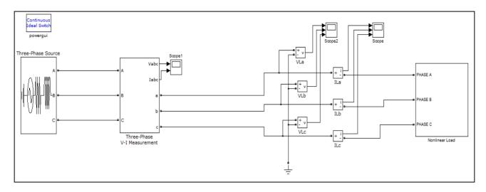
Figure 3 Simulation circuit without APF
