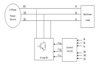
Figure 1 Shunt APF in 3 phase system
