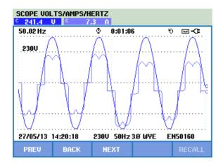
Figure 14 Voltage and current waveform for phase c
