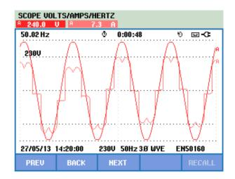
Figure 12 Voltage and current waveform for phase a
