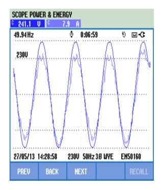
Figure 13 Voltage and current waveform for phase c
