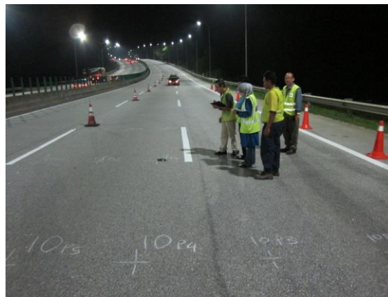
Figure 4: Lux measurement at site.
