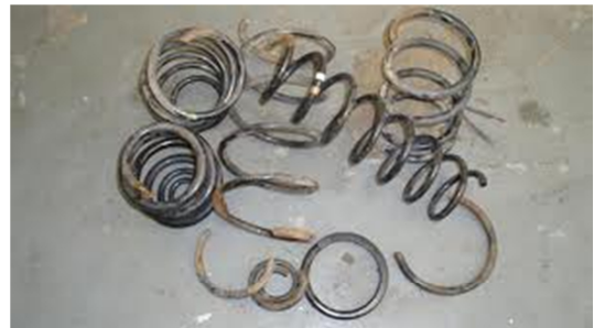
Fig. 2: Failed steel springs
