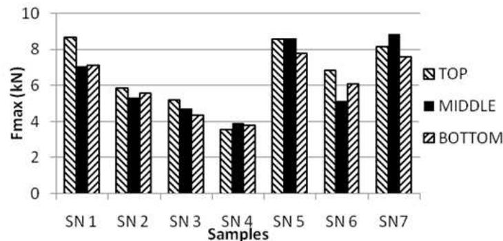
Figure 2: Maximum tensile force at break for all specimens.
