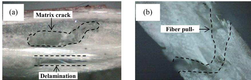
Figure 5: Optical microscope observation at fracture specimen after tensile testing (a) delamination and matrix crack (b) fiber pull-out.
