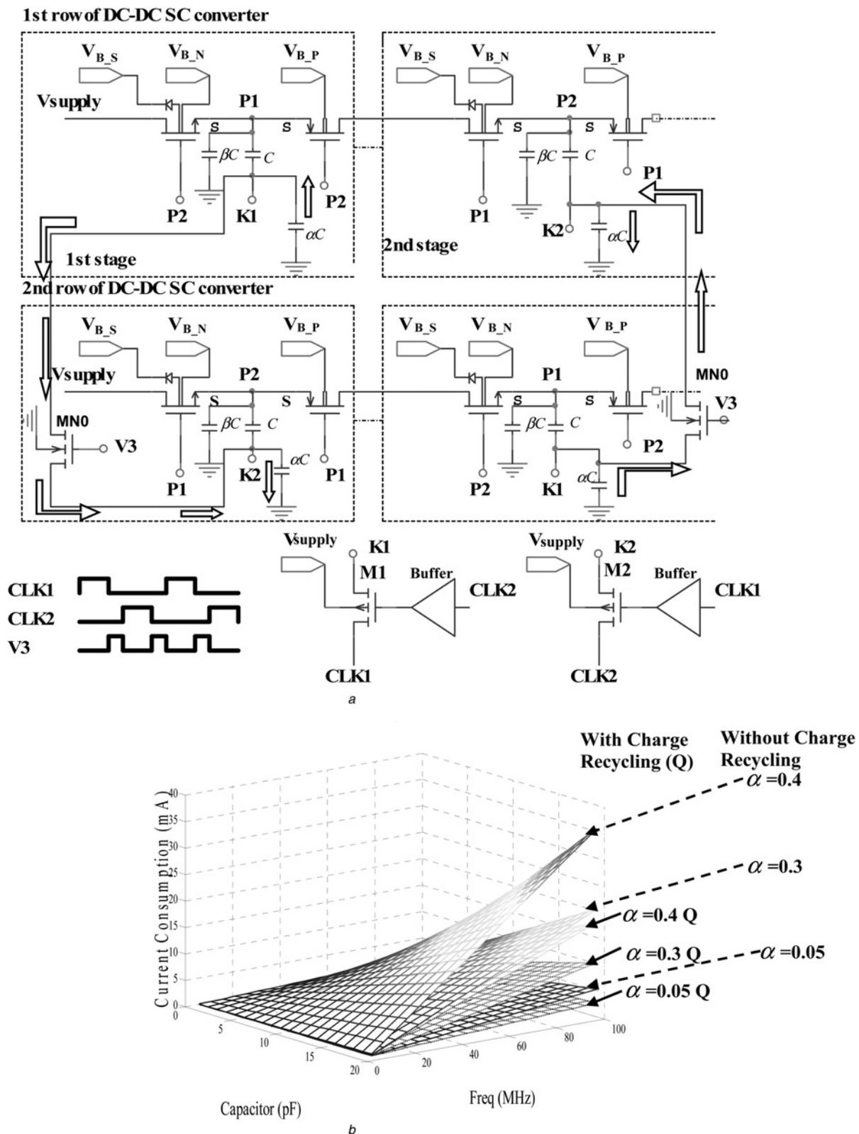
**Fig. 8** Charge recycling technique in the SC DC-DC converter
