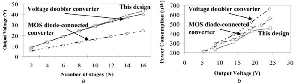
**Fig. 11** Simulation results of the improved HV SC DC-DC converter compared with the standard MOS diode-connected converter and the voltage-doubler converter, with  $0.935 \text{ pF}$  per stage at  $25 \text{ MHz}$ , in terms
