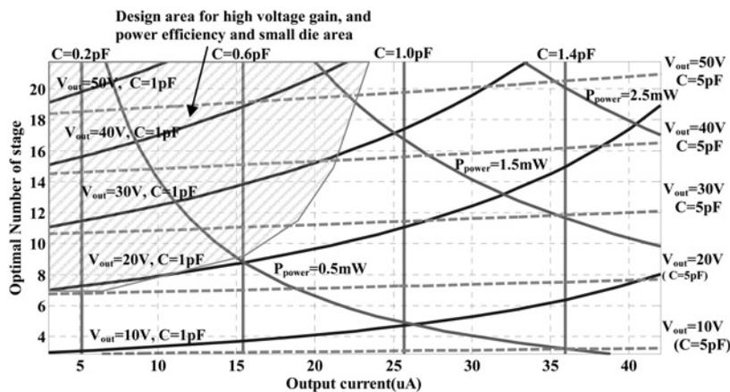
**Fig. 7** Design area of an SC DC-DC converter with an operating frequency of  $f=25$  MHz, with the assumption that parasitic capacitance loss of  $\alpha=0.4$ , and a constant threshold voltage of 0.7 V from the transistors
