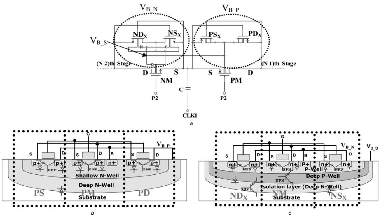
Fig. 3 Single stage of SC DC-DC converter with the adaptive bulk-biasing circuit
