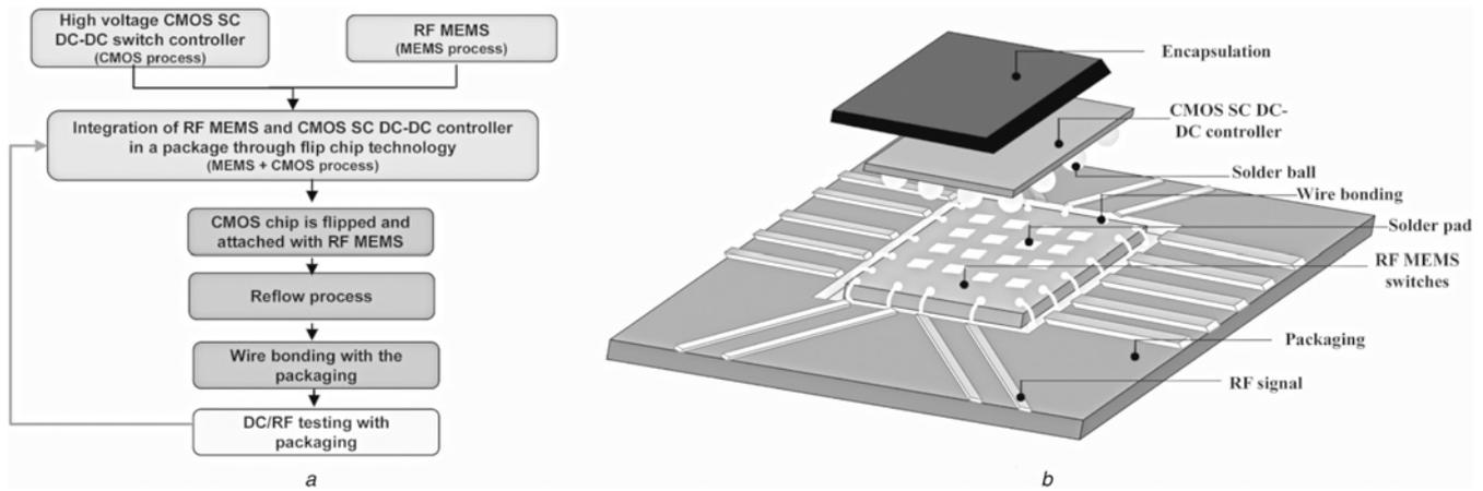
**Fig. 14** Integration of RF MEMS switches with the HV SC DC-DC converter in a single package
