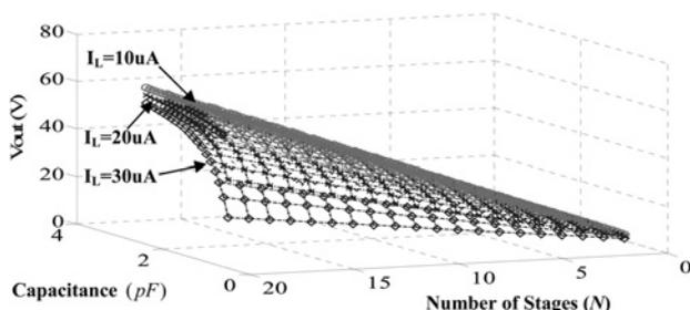
**Fig. 5** Output voltage of an ideal SC converter (without loss) operating at 25 MHz for up to 20 number of stages ( $N$ ), and three different output currents ( $I_L$ )
