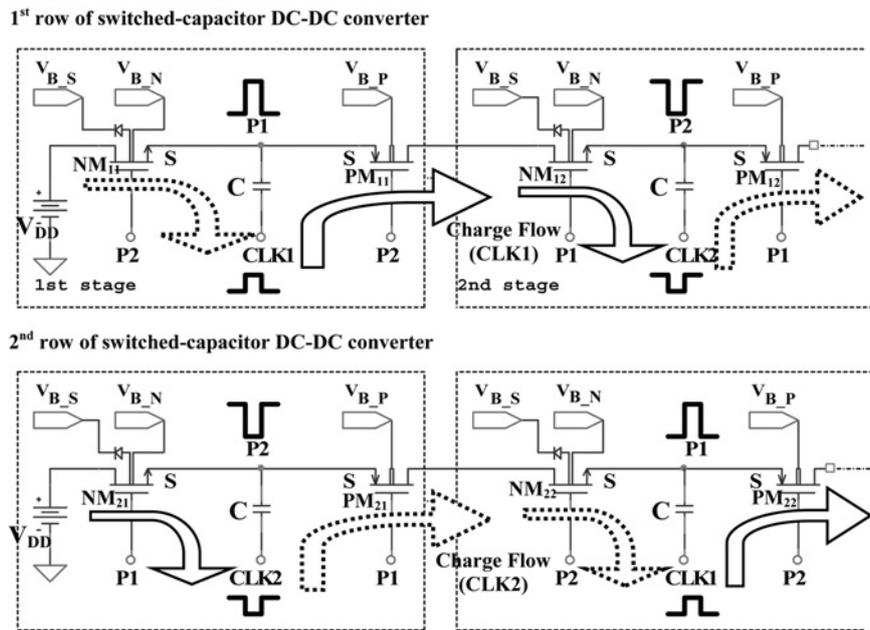
Fig. 2 Circuit diagram of an interleave structure linear voltage gain SC DC-DC Converter
