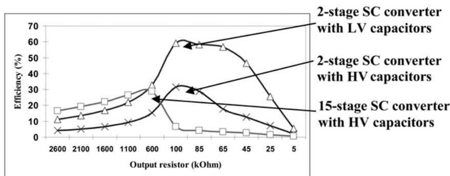
**Fig. 12** Efficiencies of a 2-stage and a 15-stage SC DC-DC converters using HV capacitors compare with a 2-stage SC converter using LV capacitors
