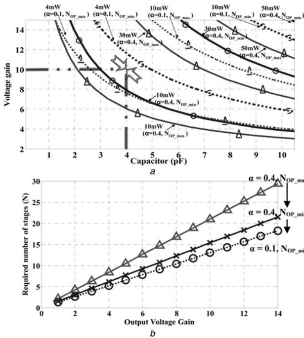
**Fig. 6** Comparison of power consumption and voltage gain by minimising  $I_L(O)$  and maximising  $I_L(\Delta)$  design
