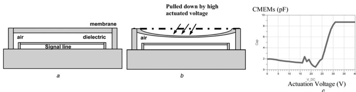
**Fig. 1** Operation of RF MEMS
