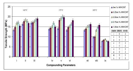
Fig.3. Tensile Strength of PP-MWCNTs Composites Compounded at 165-185°C at Various Roller Rotor Speed of Internal Mixer.
