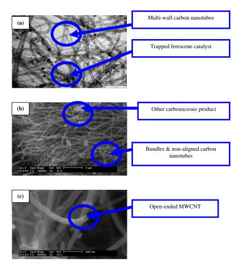
Fig.2. Morphology Observation of Synthesised MWCNTs through TEM & SEM.
