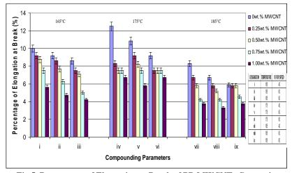
Fig.5. Percentages of Elongation at Break of PP-MWCNTs Composites Compounded at 165-185°C at Various Roller Rotor Speed of Internal Mixer.
