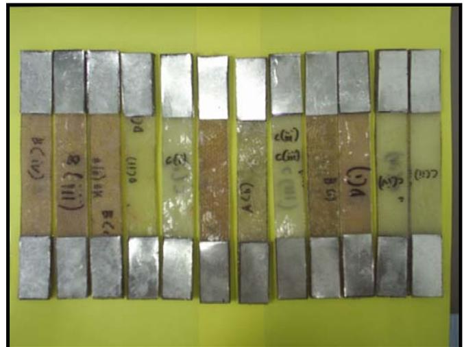
Fig. 1. Specimen for tensile test ASTM D3039
