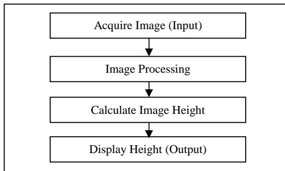
Fig 1: Block Diagram For Product Measurement
