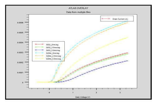
**Fig. 2:**  $I_D$  versus  $V_G$  - Comparison between SiO<sub>2</sub> and Si<sub>3</sub>N<sub>4</sub> dielectric material across thickness.
