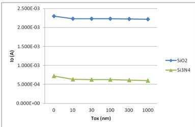
Fig. 11:  $I_D$  versus stress time – Comparison between  $SiO_2$  and  $Si_3N_4$
