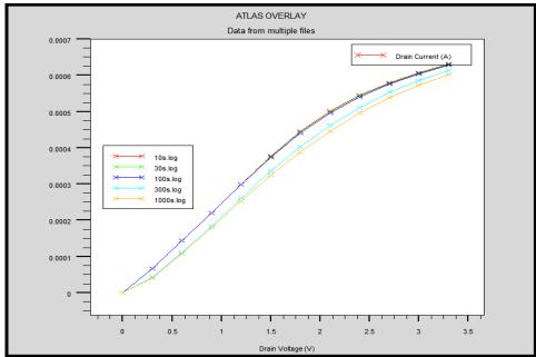
Fig. 8:  $I_D$  versus  $V_D$  – Drain current degradation.
