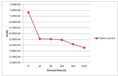
**Fig. 9:**  $I_D$  versus stress time.
