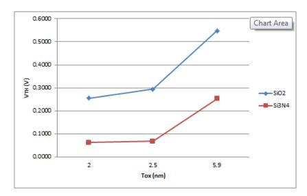
Fig. 3:  $V_{TH}$  versus  $t_{ox}$  - Comparison between SiO<sub>2</sub> and Si<sub>3</sub>N<sub>4</sub> dielectric material across thickness.
