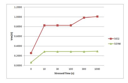
Fig. 10:  $V_{TH}$  versus stress time – Comparison between SiO<sub>2</sub> and S<sub>i3</sub>N<sub>4</sub>
