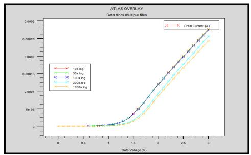
**Fig. 6:**  $I_D$  versus  $V_G$ - Threshold voltage shift across stressing time
