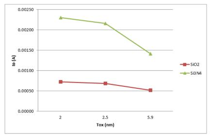
Fig. 5:  $I_D$  versus  $t_{ox}$  – Comparison between SiO<sub>2</sub> and Si<sub>3</sub>N<sub>4</sub> dielectric material across thickness.
