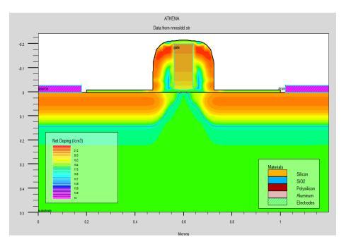
Fig. 1: Full LDD n-MOSFET structure
