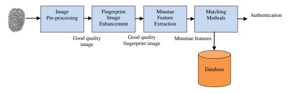
Fig 2 General Architecture of a Fingerprint Verification System
