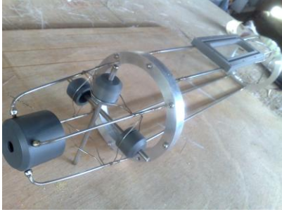
Figure 6: Skeletal Frame front view of an AUV
