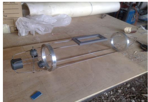
Figure 5: Skeletal Frame view side of an AUV
