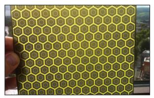
elements, so the resistive material array of elements can be applied with a uniform thickness. The resistive material itself brings a cost saving as, for the first time, the QUB team have used a low-cost high-frequency paint normally used for EM shielding of buildings.
