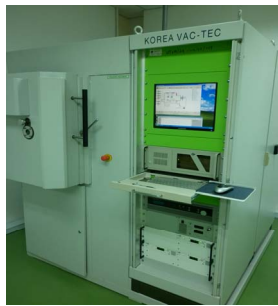
Figure 1. PVD unbalanced magnetron sputtering system VACTEC Korea model VTC PVD 1000.
