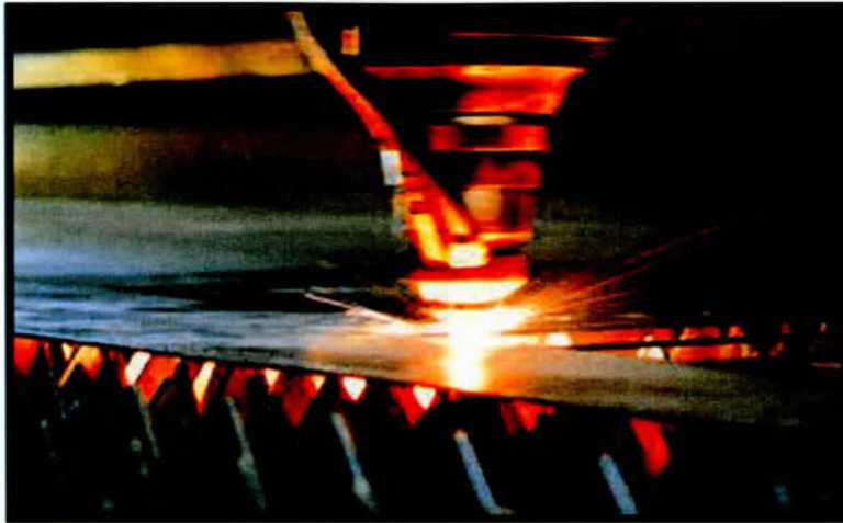
Figure 1.2 Laser Bevel Head Bevel Head for Vertical and Bevel Cuts From 0^{\circ} - 50^{\circ} .
