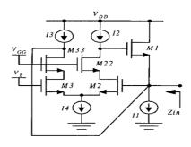
Figure 5 Double Feedback With Second Order Circuits[3]
