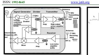
Figure 1 Block Diagram Of RF Transceiver[1]
