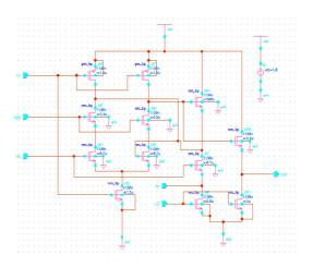
Figure 7 Schematic Of Proposed Low Noise Amplifier After Enhancement
