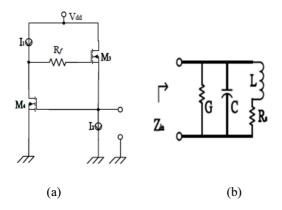
Figure 4 Active Inductor Circuit And His Equivalent Circuit[3]
