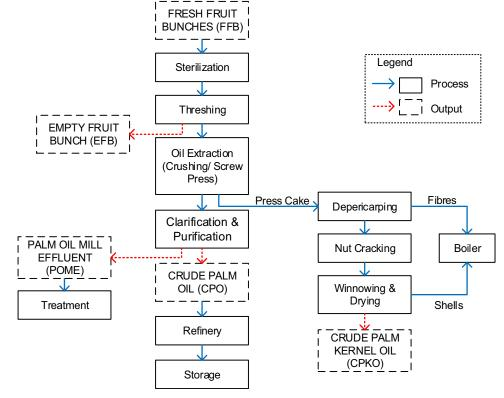
Fig. 1. Palm oil process flow.
