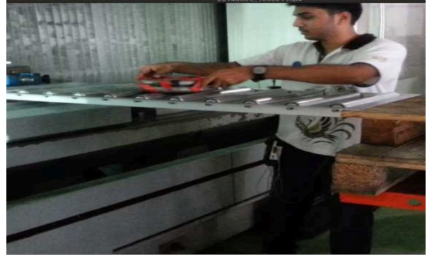
Fig. 5 Subject uses roller conveyor to push work piece to machine
