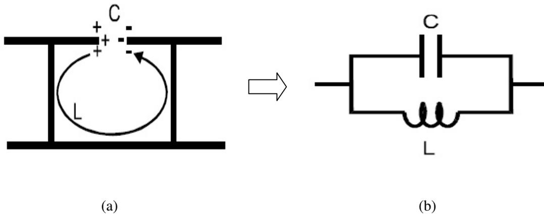
**Figure 1.2.1 : Equivalent circuit model for the high impedance surface [24]**
