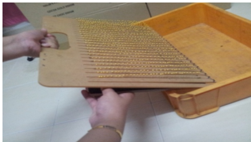
Figure 7: Step 2-Pull the jig and the pin will eject from the base into the polybin
