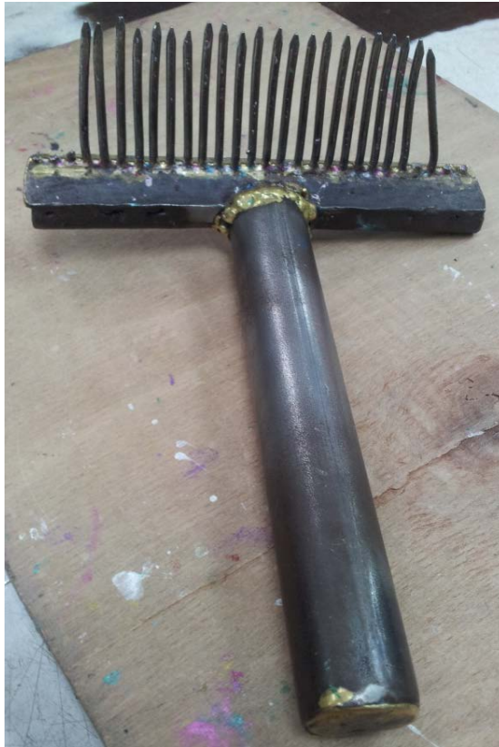
Figure 3.6: Equipment to eject pins
