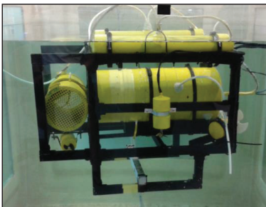
Figure 6: ROV Testing on Lab tank
