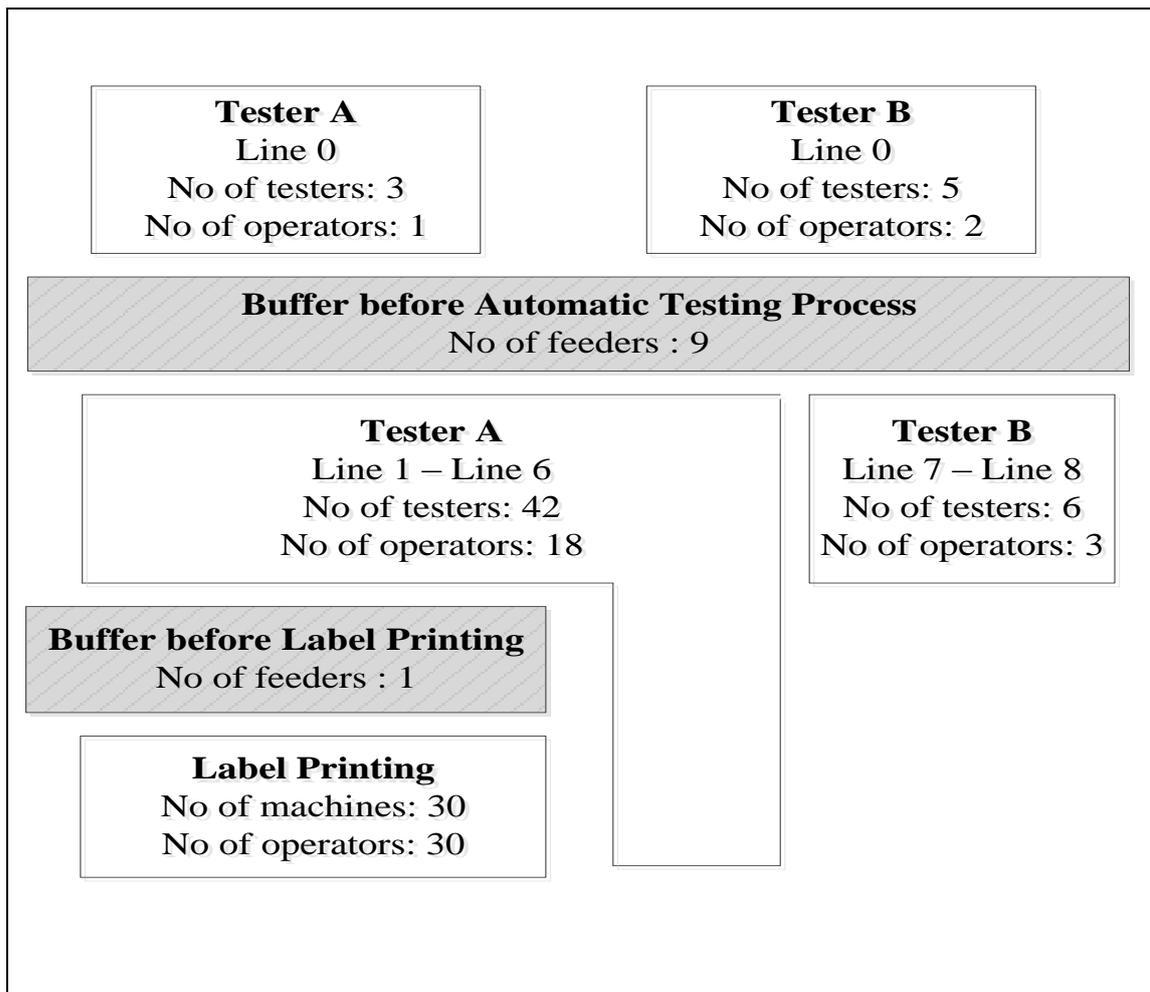
Figure 1.2 Layout of Automatic Testing and Label Printing Processes
