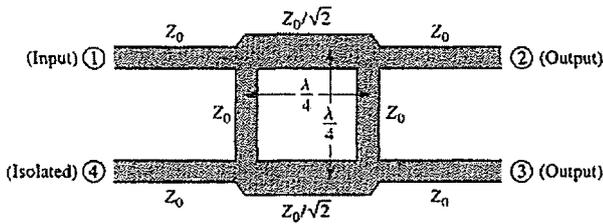
Figure 3 Geometry of branch-line coupler
