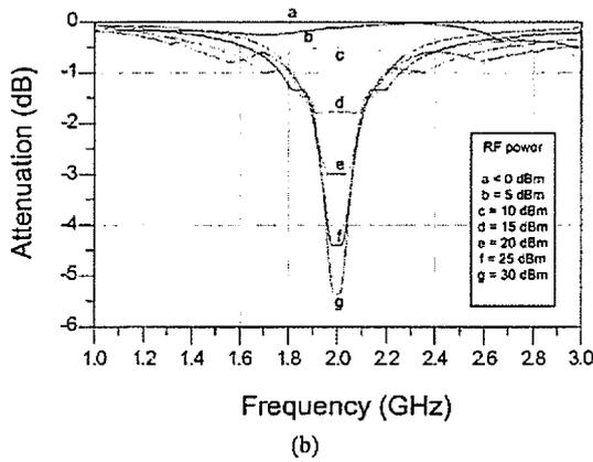
Figure 5(a): An LC bandstop filter loaded with a diode.; (b) Simulation of an LC bandstop filter loaded with a diode
