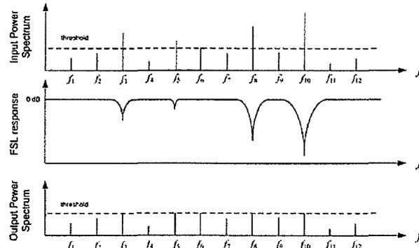
Figure 1: Basic operation of a frequency selective limiter.
