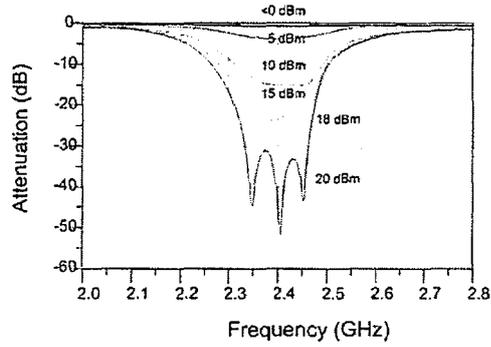
Figure 9 Simulated results of a third-order nonlinear bandstop filter.
