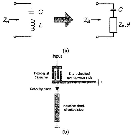
Figure 6(a): A transformation of an LC resonator to a capacitively-coupled transmission line resonator; (b) A microstrip bandstop resonator loaded with a diode
