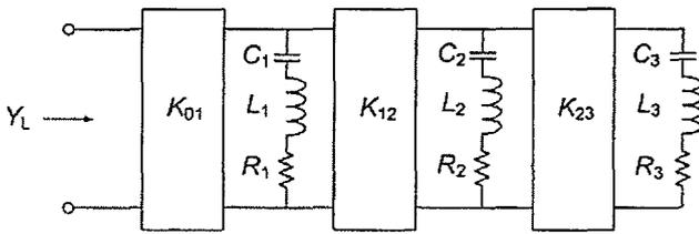
Figure 8 Lumped circuit of a third-order bandstop filter sub-network.
