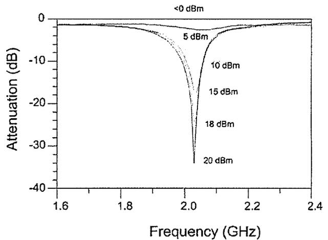
Figure 7 Simulated results of a first-order nonlinear bandstop filter
