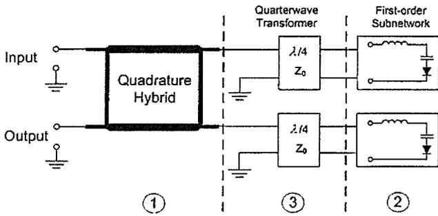
Figure 2 Circuit elements in a first-order nonlinear bandstop filter.
