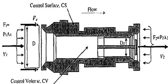
Figure 5: Cross sectional view of water nozzle
