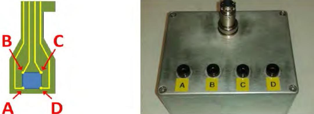
Figure 13: PCB sample board (left) and connector box (right)
