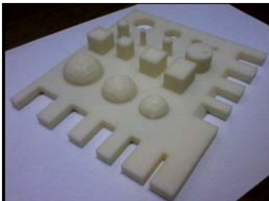
Figure-2. The FDM model of part features.
