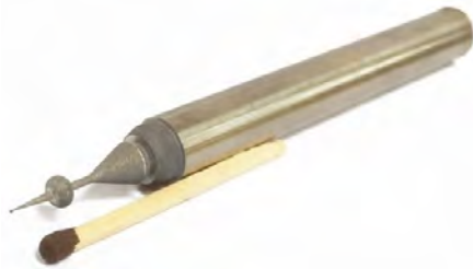
Figure 3 WEDT free- form profile machined part.
