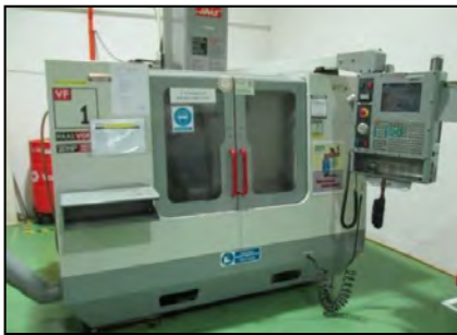
Figure 2 Three axis CNC machine used in the experiments.
