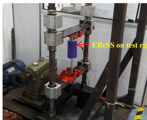
Figure 1 Test rig for the EReSS testing on laboratory.
