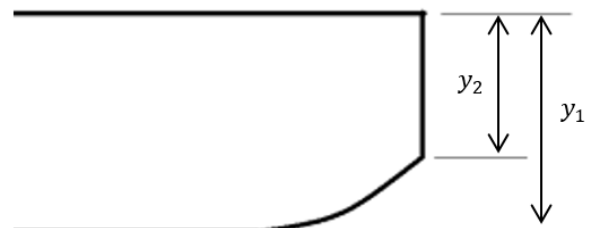
Figure 2 Method of measurement at each sample's corner
