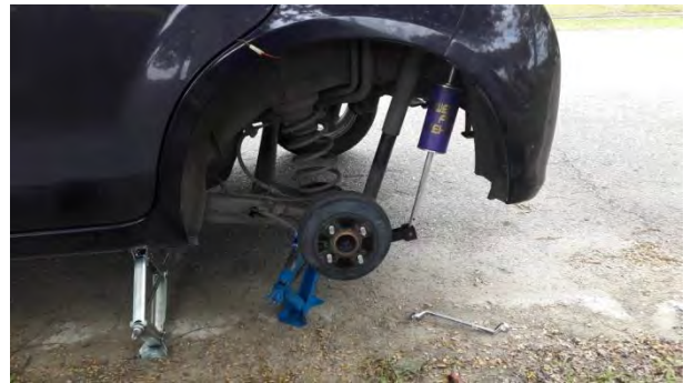
Figure 1 Regenerative system is attached to the vehicle.
