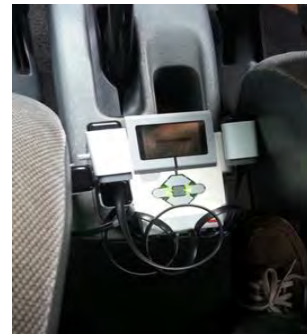
Figure 1 Lego Mindstorms DAQ and sensors.
