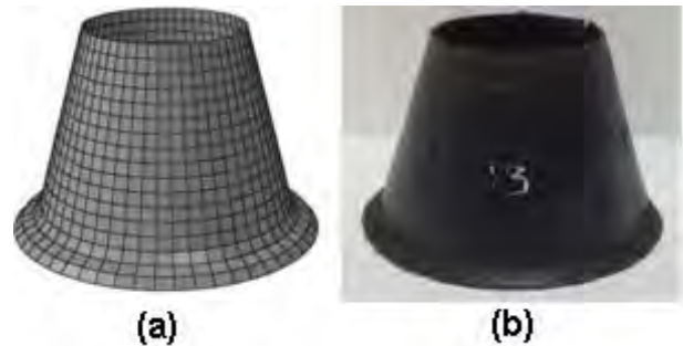
Figure 3 View of FE simulated deformed shape (Figure 3a) and collapsed cone (Figure 3b) subjected to axial compression.
