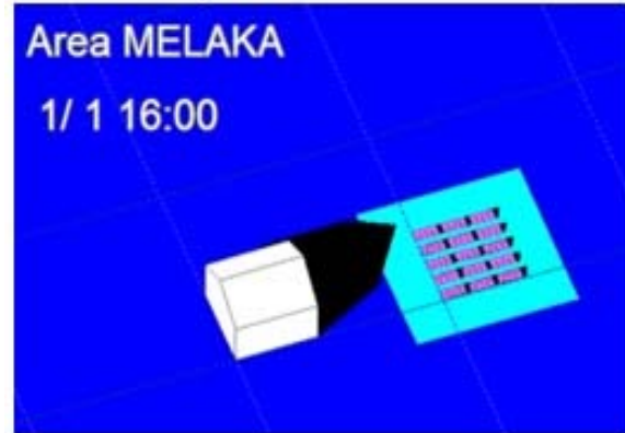
Figure-2. 20m by 20m building beside the 20m by 20m PV power plant.
