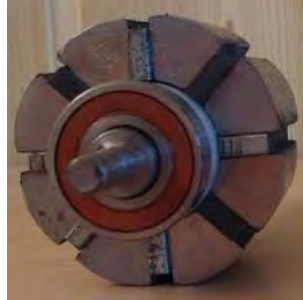
Figure 1.3: Spoke type motor construction
