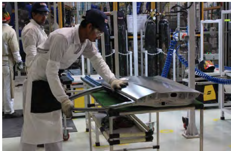
Figure 1.2 The body panel inspection by human workers
