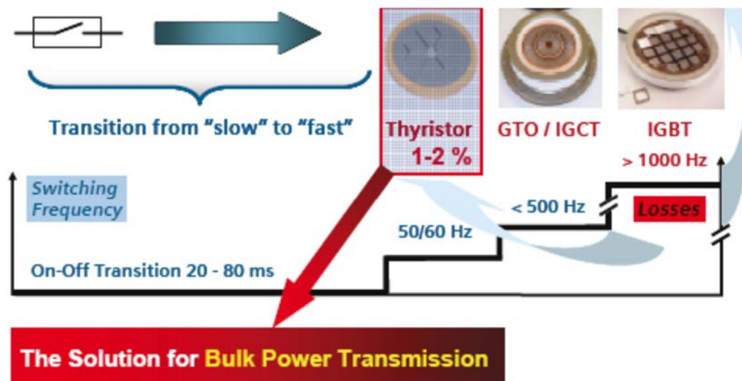
FIGURE 2.1: POWER ELECTRONICS FOR HVDC [11]
