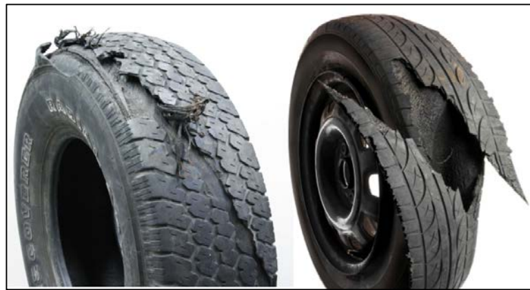
Figure 1.1 : Tyre Blowout due to Tread Separation (Willis, 2000)
