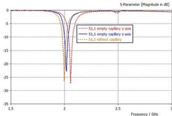
**Figure-5.** Frequency shifting of different position capillary.
