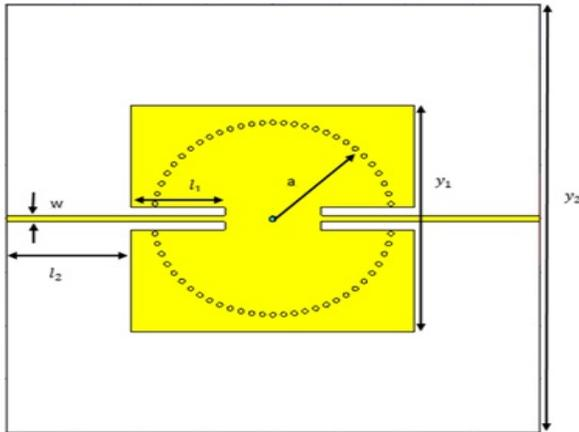
Figure-1. Resonator sensor dimensions structure design.
