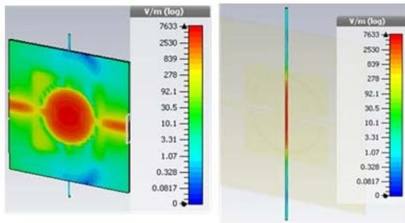
**Figure-6.** The y-axis position of capillary and the amount of electric flux on sensing area inside capillary
