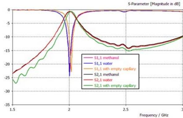
**Figure-4.** S-parameters of resonator with presence of solvents.
