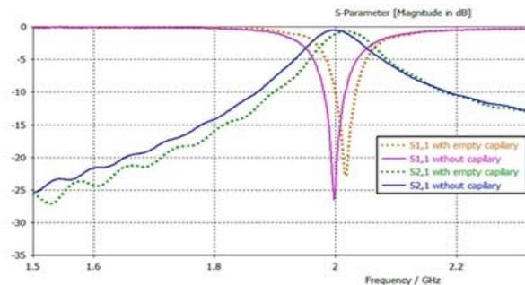
Figure-2. Insertion loss and return loss of resonator with/without empty capillary.
