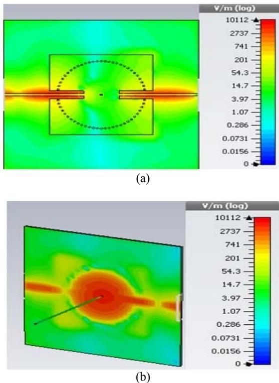
**Figure-3.** Electric fields distribution of circular SIW sensor for the whole structure. (a) Top view (b) view on substrate.
