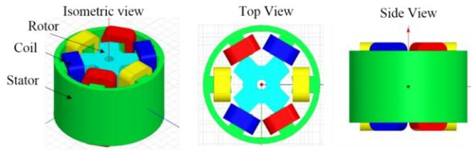
Figure 6 Structure of S:R = 6:4 poles ratio actuator
