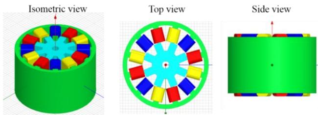
Fig. 7. Structure of S:R = 12:8 poles ratio actuator
