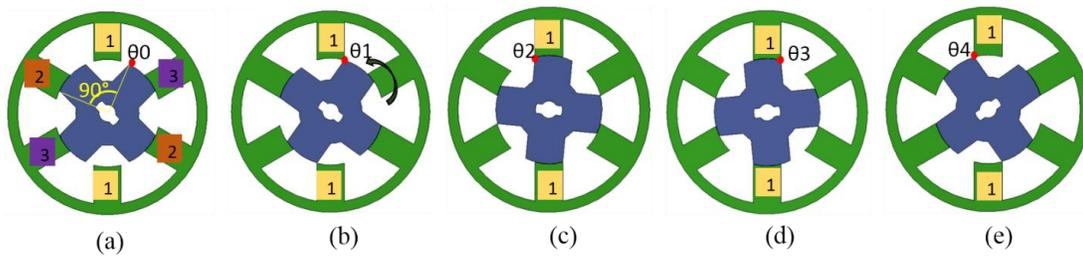
Fig. 3. Rotor position to derive the inductance profile
