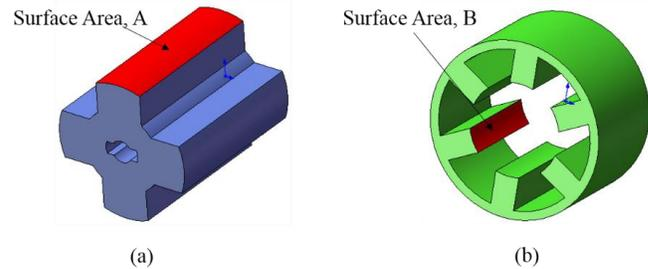
Fig. 5. Area of the active region for (a) rotor and (b) stator
