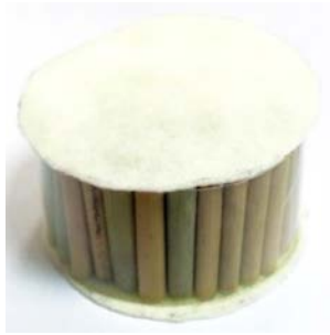
Fig. 8. Front and back surfaces of the bamboo absorber covered with fabric.
