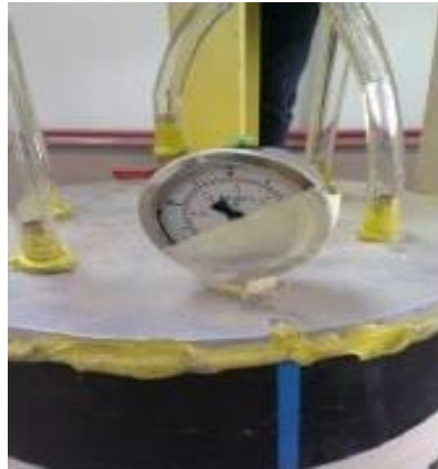
Figure 3. Drop test is carried out to identify leaks in fabrication.
