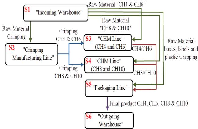
Figure 3: Process model of CHM factory floor [4, 23]
