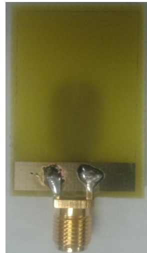
Figure 4. Back view of Spanar antenna.
