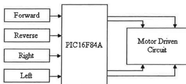
**Fig. 1. Block Diagram of PIC16F84A Operation**
