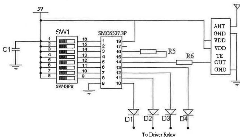
Fig. 3. Receiver Schematic
