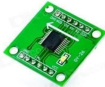
Figure 4: Magneto resistive sensor
