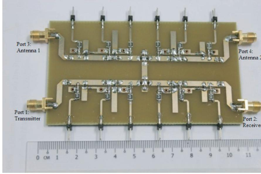
**Figure 8.** Prototype of the proposed selectable DPDT switch with switchable transmission line stub resonators, (dimension: 104 mm × 54 mm).
