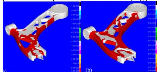
Fig. 12: Longitudinal fatigue test (a) and lateral fatigue test (b) analysis results
