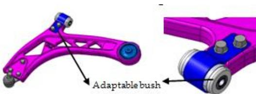
Fig. 10: Final design of aluminium cast FLCA with adaptable bush
