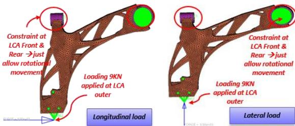
Fig. 5: Longitudinal and lateral fatigue analysis model setup
