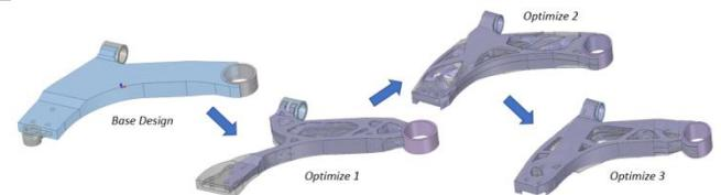
Fig. 3: Topology optimization process of aluminum cast FLCA
