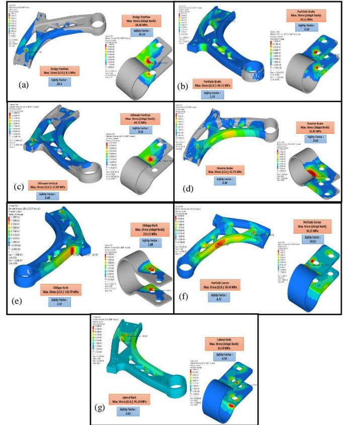
Fig. 11: Structural strength results for final design
