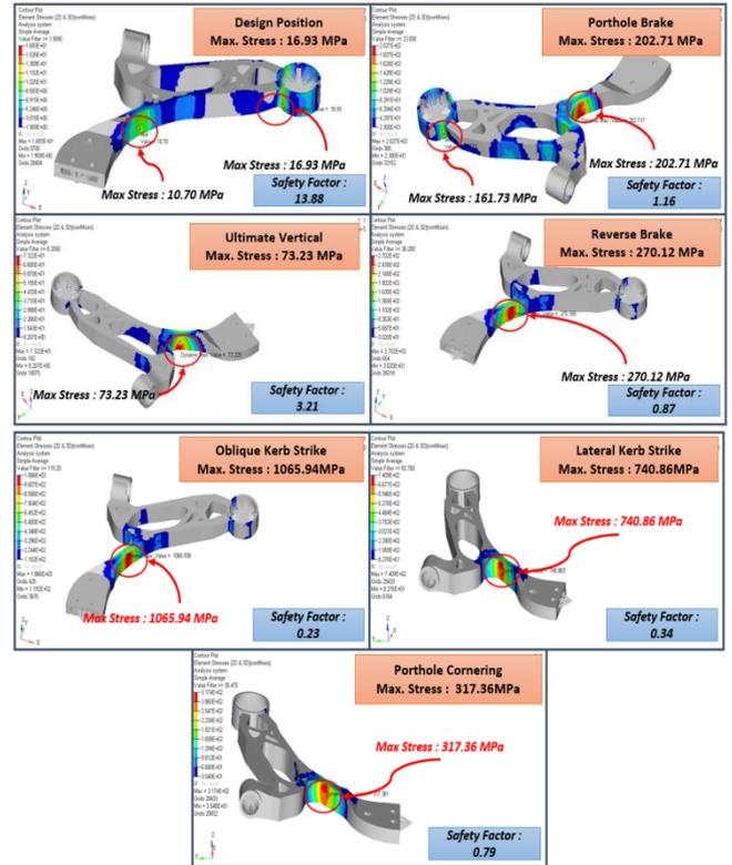
Fig. 7: Structural strength results for design iteration 1
