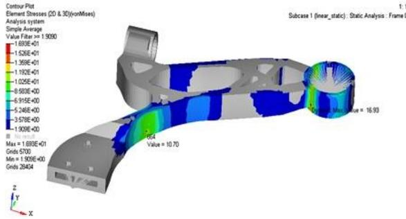
Fig. 4: Structural strength analysis using Hypermesh software
