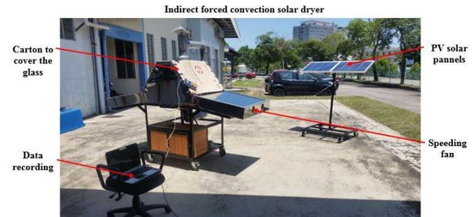
Fig. 16. The configuration of Indirect forced convection solar dryer.
