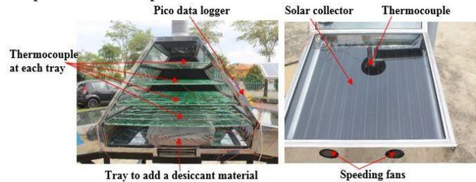
Fig. 3. Thermocouples locations in the dryer.
