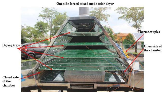
Fig. 13. Configuration of the mixed mode solar dryer with forced convection from one side of the chamber only
