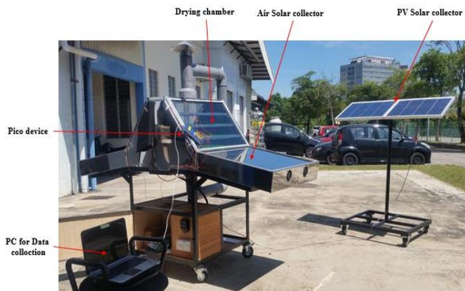
Fig. 2. Configuration of the experimental set up
