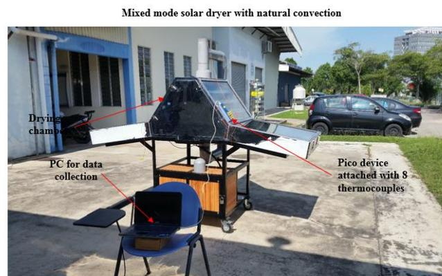
Fig. 4 .Configuration of the mixed mode solar dryer with natural convection.
