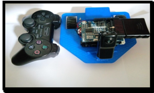
Fig. 8: Hardware of security robot
