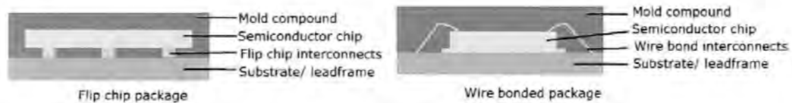
Figure 2.1: Comparison between flip chip and wire bond package
