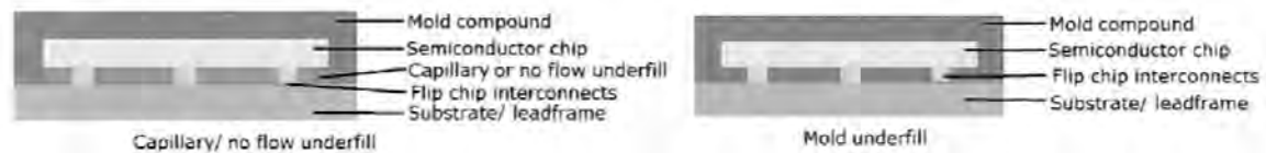
Figure 2.2: Comparison between capillary / no flow underfill with mold underfill
