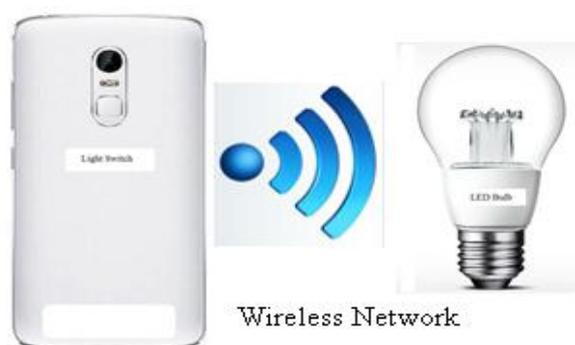
**Figure 1:** Device to Device communications via Bluetooth, Z-Wave or ZigBee can be set up to switch on/off a light bulb [13]
