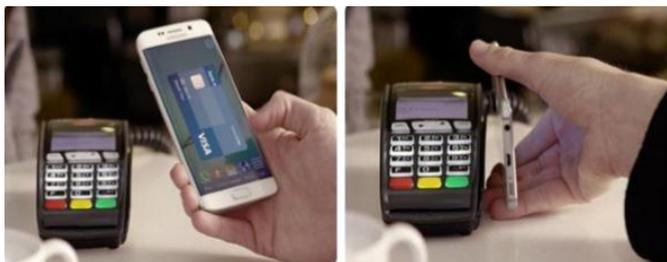
**Figure 6:** A payment swiping on the NFC terminal on the left or a touch on the MST terminal
