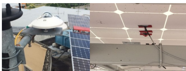
Fig.14. Pyranometer CM 11 (left) and CS220 surface-mount thermocouple (right)
