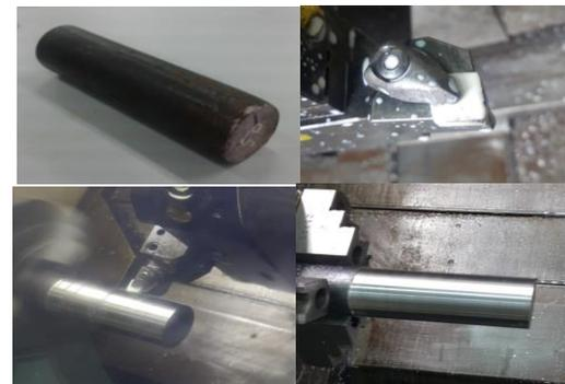
**Fig. 3.** (a) Workpiece material of AISI 1045 (b) Alumina cutting tool on tool holder (c) Straight turning operation (d) machined surface of AISI 1045
