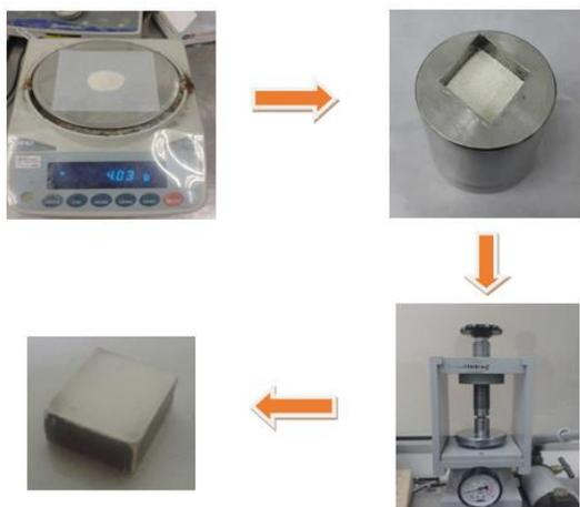
**Fig. 1.** Pre-compaction process of alumina powder into compacted green body
