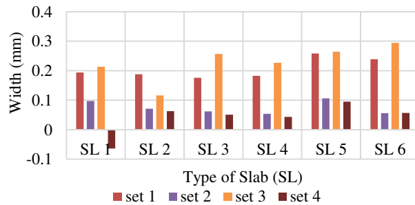
Figure-5. Deviation of width of Slab (SL) for Mendel Max 3D printer using PLA material.
