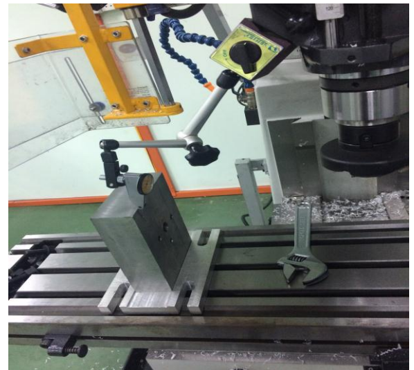
Figure 4: Allignment process (Clamp lever assemble)
