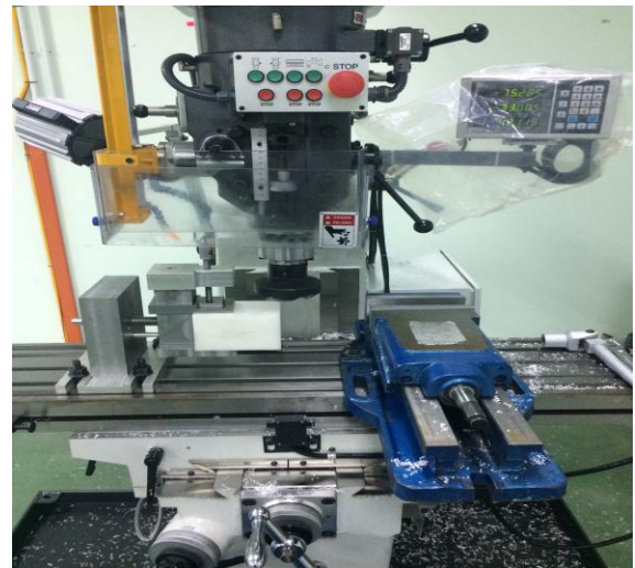
Figure 8: Work piece clamp using flexible clamping
