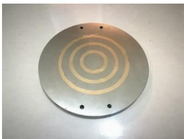
Figure-12. Brass is fitted into the slot.
