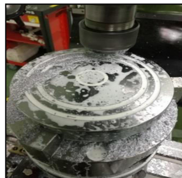
Figure-8. Slots in progress using the milling machine.
