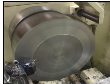
Figure-7. Facing process on the raw material.
